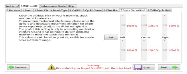
Here is where you set your swash movement limits so that there is no mechanical binding. If binding occurs use the sliders or arrows to limit the movement of the swash servos so that there is no mechanical interference. Once done click on Save and Next.
