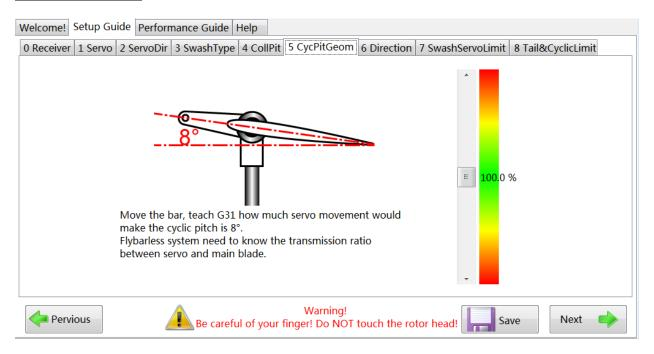
This step teaches the BlackWidow how much servo movement is required to achieve 8 degrees of pitch. With the blades running the length of the helicopter and the pitch gauge on the blade, move either the up or down arrow until your pitch gauge reads 8 degrees of pitch. Once you are at 8 degrees click on Save and then Next.
