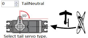
Fix the servo arm. Servo arm should be perpendicular to tail linkage rod.
