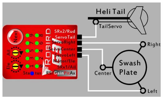
[ServoLeft, ServoCenter, ServoRight] each connect to [Left, Center, Right] 3 swash plate servos. ServoTail connect to tail servo.
