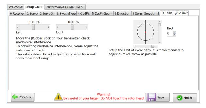
This is where you set your range of movement for your tail so that there is no binding. Use the slider to increase as needed for the left and right limits. On the right side of the screen you can reduce the amount of movement
