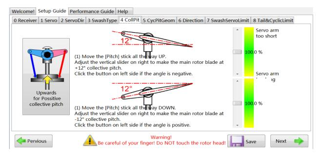
Place the main blades so that they are running the length of the helicopter. Move your collective pitch control to its full up position. Use your pitch gauge to determine how much pitch the system has. Click on the Up or Down arrows as needed to adjust the pitch of the blade until you have 12 degrees of positive pitch. Then move the collective pitch control to its full
