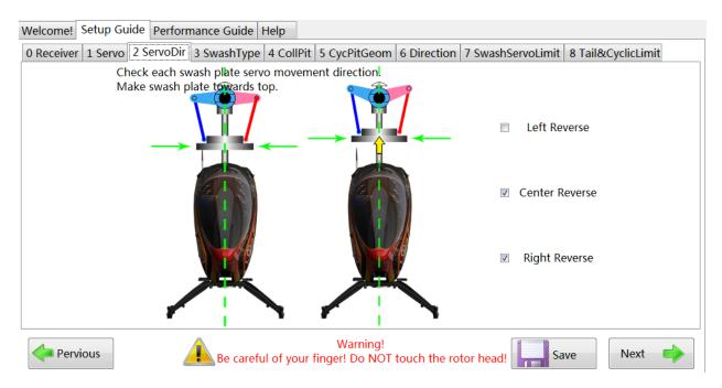
On this step you will select your servo direction. You will have to select save then disconnect the cable from the BlackWidow unit to verify if the servos are moving the correct direction. You will come back to this section several times until the swash is moving in the proper directions. Once moving in the proper direction click on Save and then Next.
