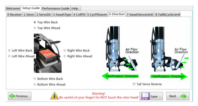
Click on the radio button that best matches how your BlackWidow is mounted on the helicopter. You may have to unplug the cable from the BlackWidow unit to verify the direction of the tail blades. Use the diagram on the screen as your guide. If it is NOT moving in the proper direction put a check in the Tail Servo Reverse box. While verifying this step you will also want to verify that the stick inputs for the tail are also setup correctly.
