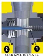
The low-speed needle (1) simply regulates how much fuel flows from the inlet (2) at lower engine speeds. At full throttle, however, the low-speed needle is fully maximum flow.
