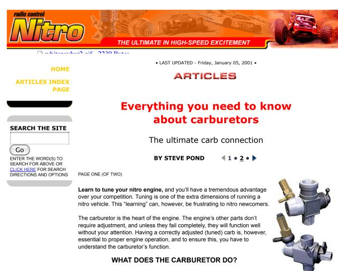
The carburetor simply regulates the flow of air and fuel (air/fuel mixture) through the engine in a way that optimizes performance throughout the engine's rpm and load range.
