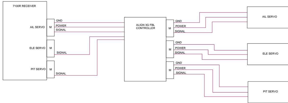
THIS IS HOW I AM GOING TO GET AROUND THE ALIGN WIRING BLUNDER. I AM GOING TO CREATE A COUPLE OF "Y" CABLES THAT ARE FEMALE TO 2 MALES THAT I CAN THEN PLUG INTO THE ALIGN FLYBARLESS CONTROLLER AND THEN RUN A JUMPER FROM THE OTHER MALE CONNECTOR WHICH WOULD CONSIST OF A FEMALE PLUG ON ONE END AND REMOVING THE PINS FROM THE MALE PLUG ON THE OTHER END AND INSTALLING THEM INTO THE MALE CONNECTOR FROM THE FLYBARLESS CONTROLLER TO THE RECEIVER.
